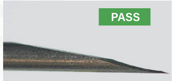
Magnified image on the Acumen AI of a good medical needle
