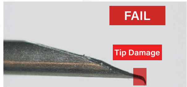
Magnified image on the Acumen AI of a bad medical needle
