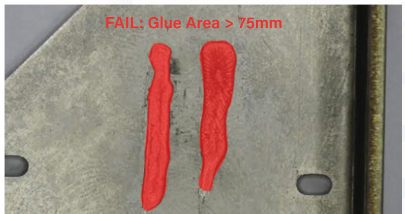
Magnified image on the Acumen AI of glue detection on an automotive part
