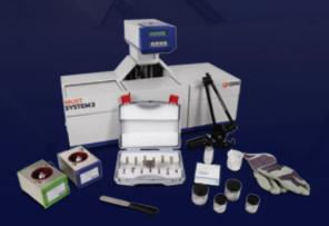
The MUST 3 sets the standard - it performs solderability testing in accordance with all major international standards and comprises everything necessary for all forms of solderability tests.
