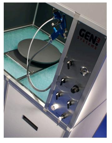
If the semi-automatic foot control for the turntable indexing system is adopted then this is connected to the manifold. The operator passes the spray gun at an angle of  $45^\circ$  over the PCAs which are supported on spigots that are mounted on the turntable.
