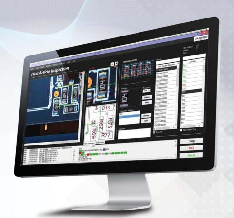
First Article Inspection is the process of independent verification of the new product to confirm that the specifications and design requirements have been properly implemented before starting a mass production.
