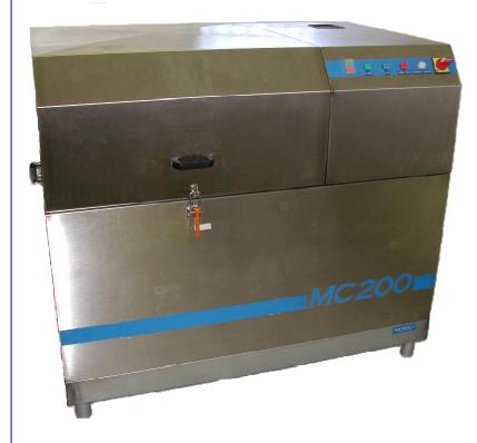
Specially designed to enhance ATRON<sup>®</sup> SP200, MC200 is based on spray in air technology. Parts are placed into a stainless steel basket, and submitted to the superior cleaning performance of high pressure sprayer. They are perfectly cleaned in just a few minutes.
