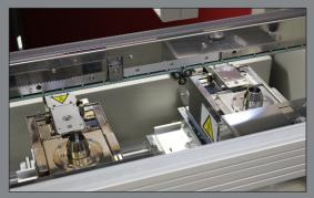
TWIN INDEPENDENT SOLDER BATHS Solder baths operating on independent X, Y & Z axis for rapid production throughput
