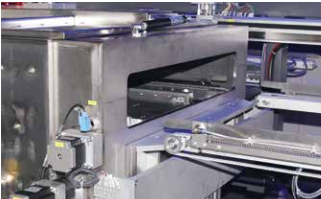
Condensox-Line cooling chamber
