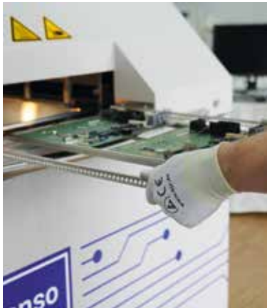
Inserting the workpiece carrier into the CondensoXC process chamber
