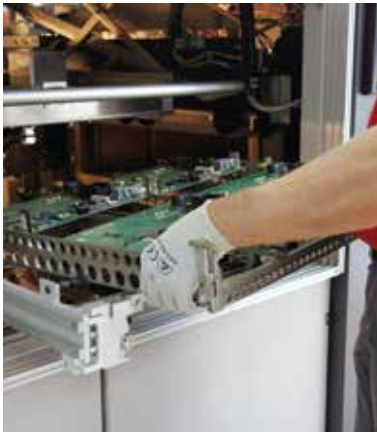
Changing the workpiece carrier with the CondensoXS
