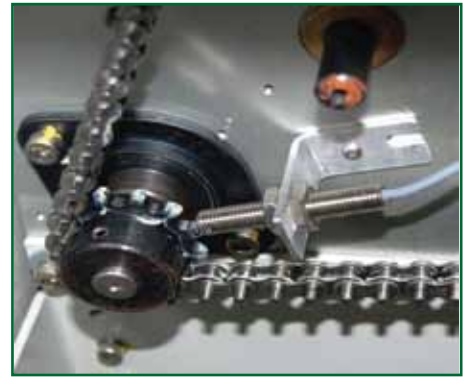
The APS system incorporates independent sensing and verification of machine conveyor speed.
